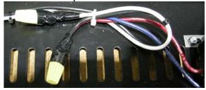
4. Run the wire along back of base and attach it to the base of the charger by using cable ties.
