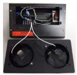
3. Screw in the adapter plate to the base.
