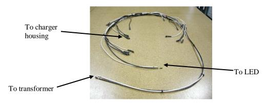
2. On a 48-unit rack, only one of the wiring harness will require the end connection to the LED. On the other 3 wiring harnesses, terminate the wires using Marrettes.
